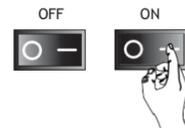
**C** After installing the software, locate the power switch on the lower right rear side of the scanner. Make sure the scanner is TURNED OFF. Plug the AC adapter into an AC power source FIRST before plugging it into the scanner. Then switch power to the "ON" position.
