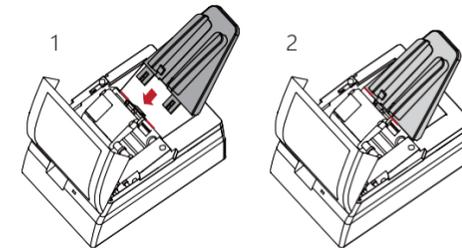
Please be sure the film feeder is inserted properly and secure before proceeding.
