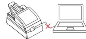
**A** DO NOT CONNECT the scanner before installing the software. If you see a "Found New Hardware" screen, click "Cancel" and disconnect the scanner.
