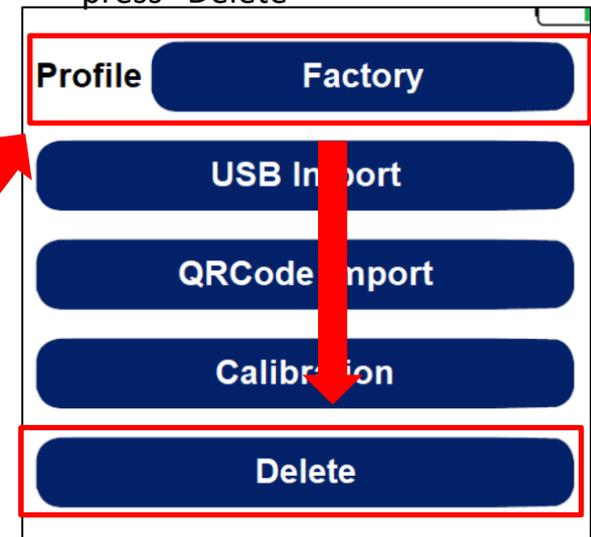
Step3. Pick a profile you would like to delete by pressing "Profile" and then press "Delete"
